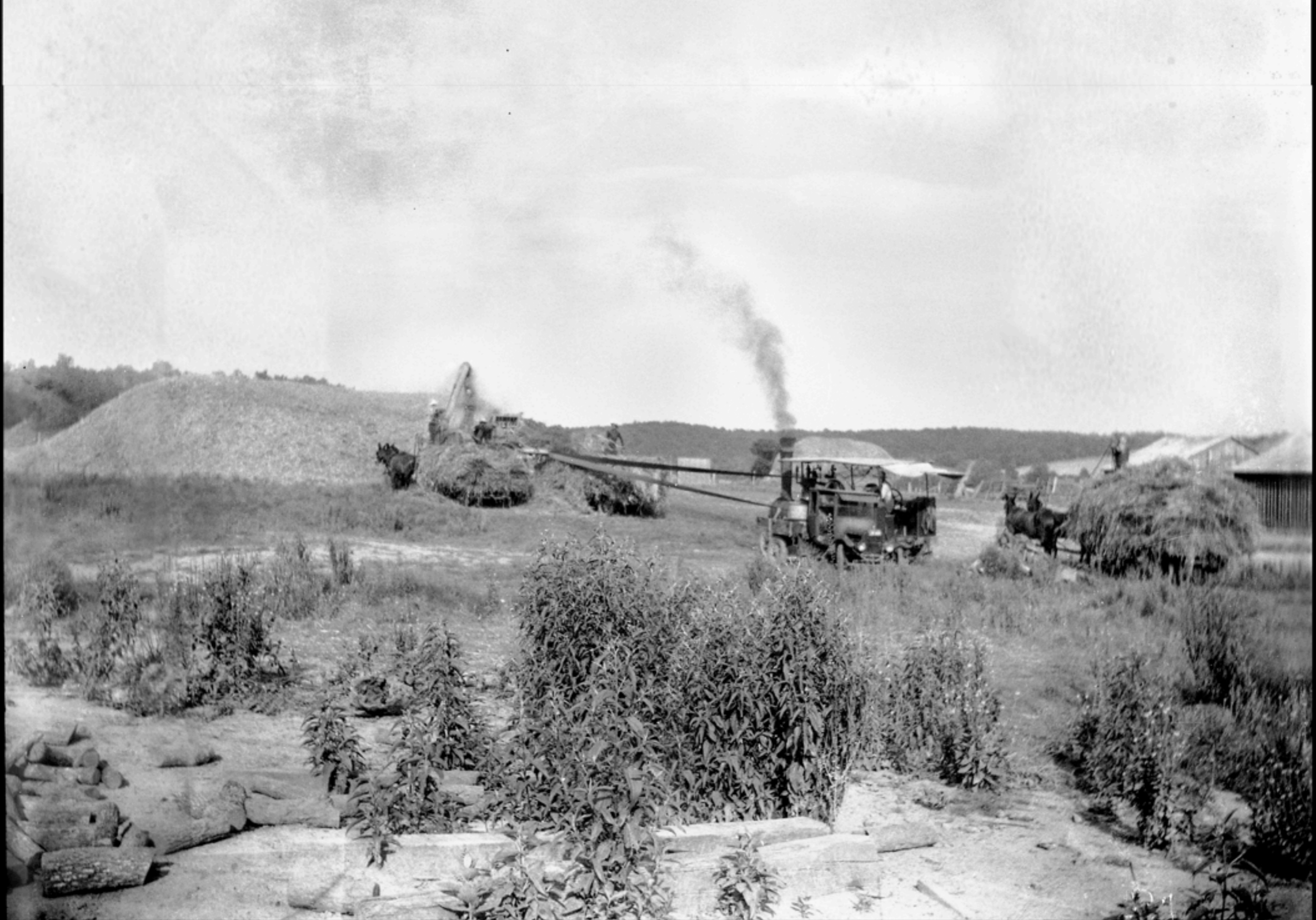
Threshing Wheat "This may have been along Femme Osage Creek. The machine was run by 2 steam engines; 3 horse- or mule-teams hauling wheat bundles. They moved from farm to farm." (EstherS; KenB)
